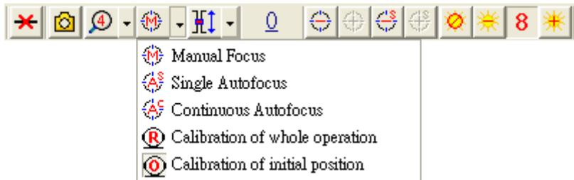
Fig 5-80 Focus ways and motor calibrate menu
