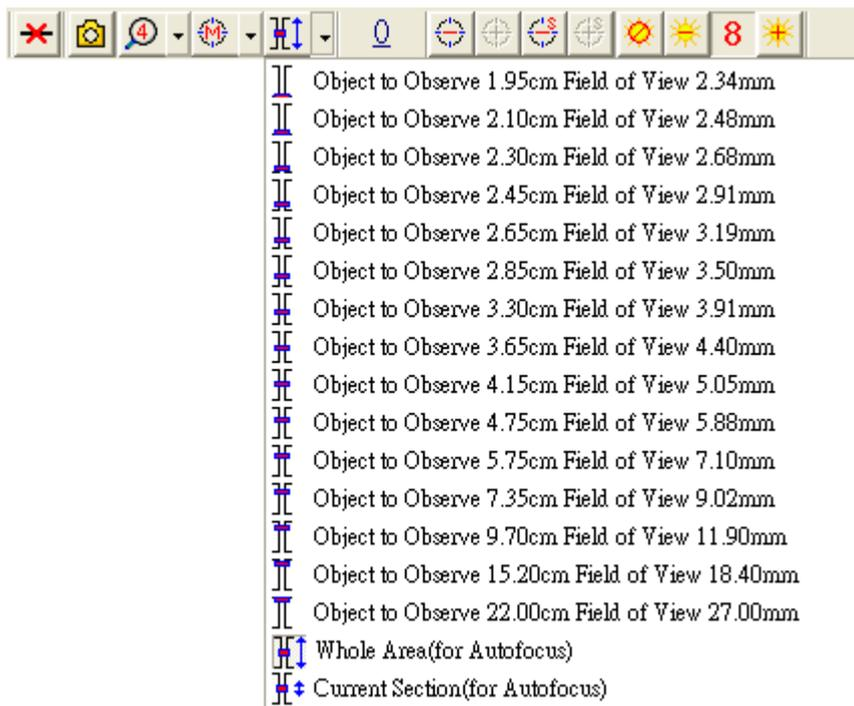
Fig 5-81 menu for Object lens 4x
