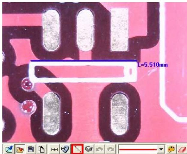
Fig 5-64 Length measurement
