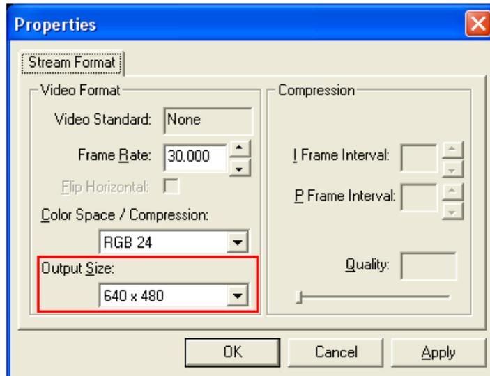
Fig.5-45 Resolution adjustment
